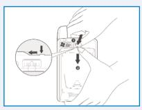
NOTE: Do not remove the battery pack for more than 30 minutes.
